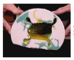
Once we've mixed equal amounts of the 610 Foam, we poured it into our mold. Because of the fine detail and multiple layers of the the turtle's head, neck, body, and feet we slushed cast the foam a couple of times to make sure we had all of the surfaces in the mold covered.
