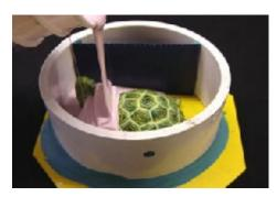
Once the mold box has been sealed, mix and pour the silicone rubber. We have chosen to use the Alumilite High Strength 3 silicone rubber because of it's low durometer and high tear strength which will aid in demolding the piece.
