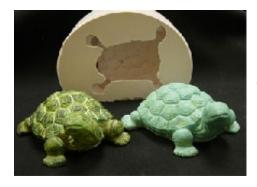
Here you can see the original turtle along side of our slush casting that was backed with the 610 Foam. The original turtle on the left used approximately 40 ounces of resin, whereas the slush cast turtle on the right used 4 ounces Alumilite resin and 3 ounces of the 610 Foam. Therefore we cut the amount of resin used from approximately 40 ounces to 7 ounces.
