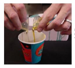
Because the outside surface is so thin and fragile, we chose to use our 610 Foam to reinforce the turtle's skin and to fill the hollow void on the inside of it's body. The 610 Foam expands 10 times the original liquid volume to give you a very durable 6 lb density foam backing.
