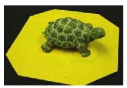
Pick a piece of plastic or wood to use as a base for the mold box. You will want the base to be approximately double the size of the piece to make sure you have room to seal the mold box thoroughly to prevent leakage.
