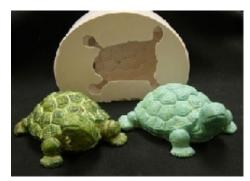
To slush cast is to pour a fraction of the amount of resin into your mold (typically of a bigger piece that has a lot of volume) and coat the sides with it by rotating the mold while the resin cures. Once the sides are coated, you can back fill the piece or leave it to be hollow.
