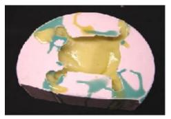
Once the foam starts to rise, we simply put the mold back down and let the foam take full form inside the turtle's hollow green slush cast. To ensure a good bond between the Alumilite resin and the 610 Foam, we recommend pouring the 610 Foam within 5-10 minutes of pouring your slush cast layer. The sooner you pour one to another, the better the bond. They would still bond to one another even after waiting a long period of time, but the sooner the better.
