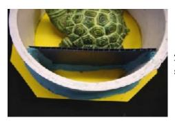
As you can see we fastened the turtle in the mold box off center to reduce the amount of wasted space. To eliminate the wasted space we cut a piece of Alumilite Corrugated Plastic and sealed it with Alumilite Synthetic Clay. We also sealed the PVC pipe to the base using the synthetic modeling clay.
