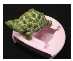
Here you can see the silicone rubber and the perfect original unaffected by the molding rubber. The moldmaking rubber will not bond to your master. Silicone rubber only bonds to other silicone rubbers. Therefore, as long as your original is not made out of a silicone rubber, the moldmaking material will not bond to it or affect the original in any way.
